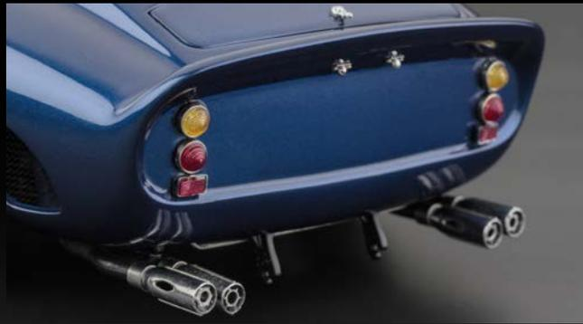
*The famous GTO-rear end with impressive racing-style tailpipe of the exhaust system.*
